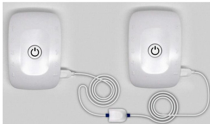
Figure 94: biosignalsplux devices connected with a sync-cable.
