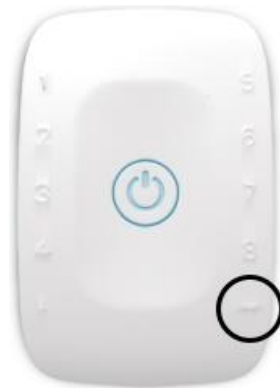
Figure 93: Digital port of the 8-channel biosignalsplux.
